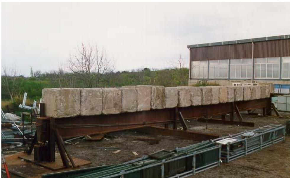
FIGURA 2-32 - VIGA DE NUNZIATA (1999) CARREGADA PARA ENSAIO
