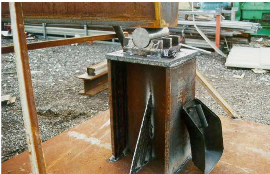
FIGURA 2-21 - DETALHE DO APOIO DA VIGA DOS ENSAIOS DE NUNZIATA, CONFIGURANDO RÓTULA NO APOIO.
