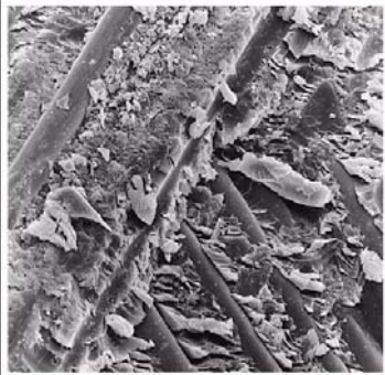
The glass fiber reinforcement in a fiberglass composite is clearly seen in a scanning electron microscope image of a fracture surface. (Courtesy of Owens-Corning Fiberglass Corporation)
